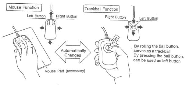
Turning over the body will automatically switch from mouse to trackball and vice versa
